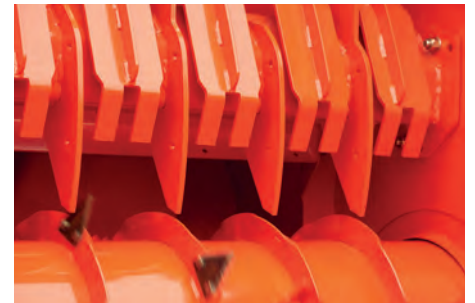
DFCS disengaged for maximum flow through the flywheel.
