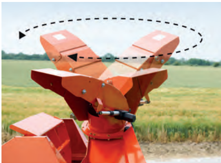
The swivel chute offers a 260° rotation of the chute.
