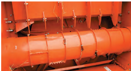
The drum-comb combination is designed for shredding straw bales in various formats.
