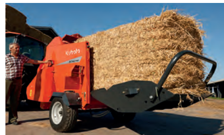
Operation of both tailgate and floor chain by using the remote control.
