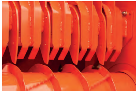
DFCS engaged to reduce the risk of blockages during loading and flywheel start up.
