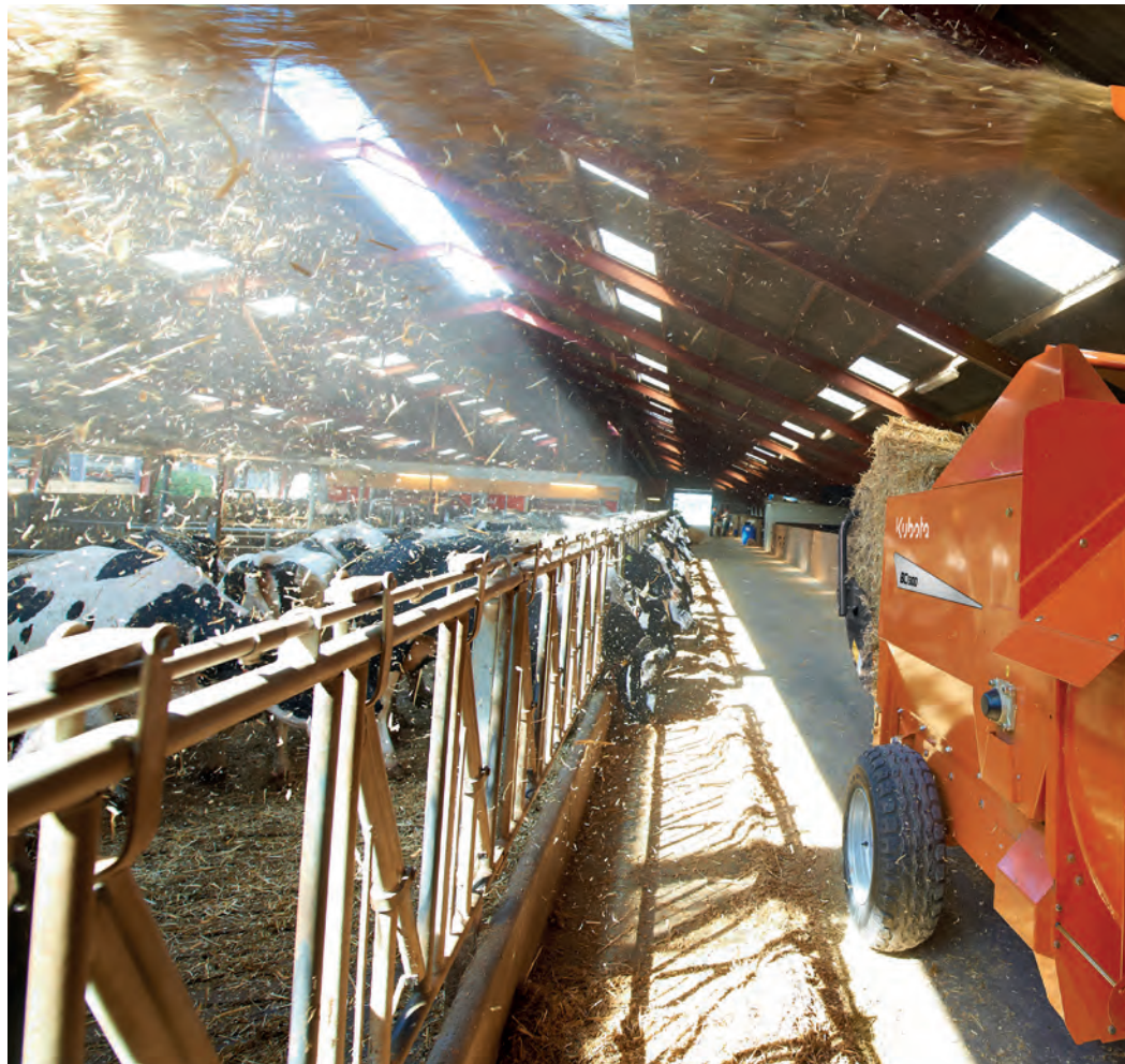
The swivel chute offers a 260° rotation of the chute.
