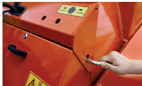
Easy shifting from bedding to feeding on the 2-speed gearbox.
