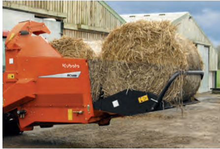
The special design of the tailgate and optional bale retainer offers the possibility to carry an extra round bale.
