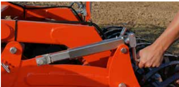
Good access and central adjustment of the levelling equipment via crank.
