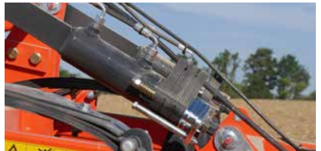
Depth control with hydraulic cylinder and spacers on CU3001.
