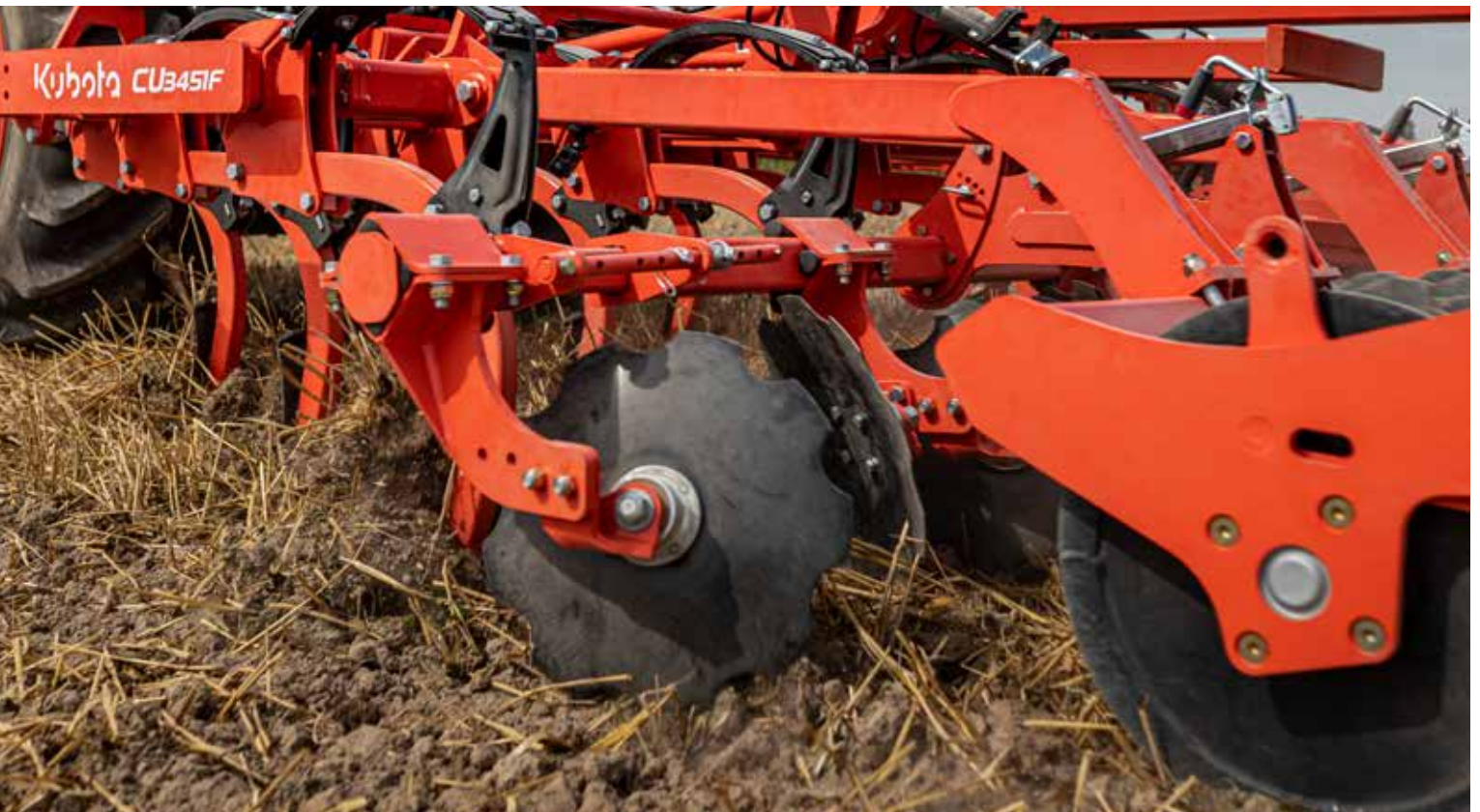
Levelling discs for heavier trash conditions.
