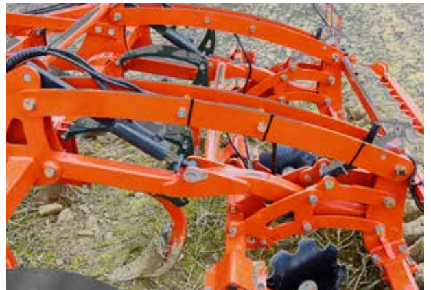
More ease of use offers the parallelogram linkage of the models with the "P". Here the working depth can be changed from the cab on the go.
