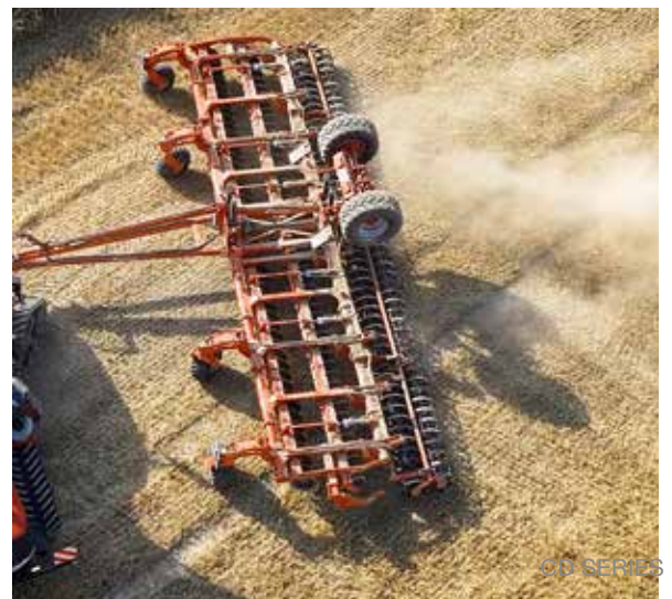
Pre-setting by scale to regulate the hub of the hydraulic cylinder in front of the depth control wheels and at the rear of the roller.
