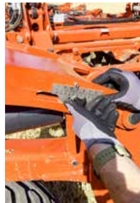
Pre-setting by scale to regulate the hub of the hydraulic cylinder in front of the depth control wheels and at the rear of the roller.
