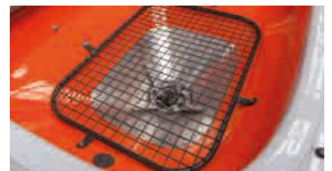
Agitator with safety grid and stainless steel insert
