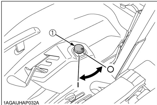
(1) PTO clutch control switch | "ON" ○ "OFF"
