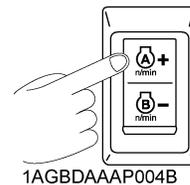
Setting RPM dual memory switch (A)
