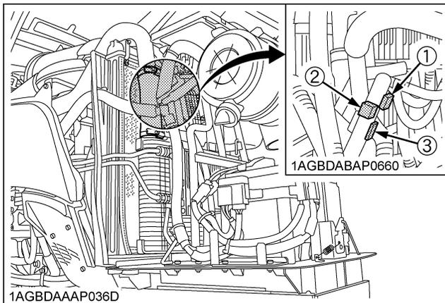
**[Oil separator Fuse] (if equipped)**
