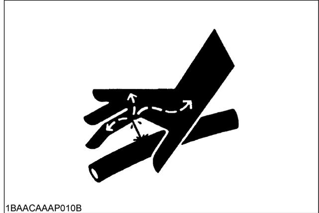
16. Fluid escaping from pinholes may be invisible. Do not use hands to search for suspected leaks; use a piece of cardboard or wood. Use of safety goggles or other eye protection is also highly recommended. If injured by escaping fluid, see a medical doctor at once. This fluid will produce gangrene or severe allergic reaction.
