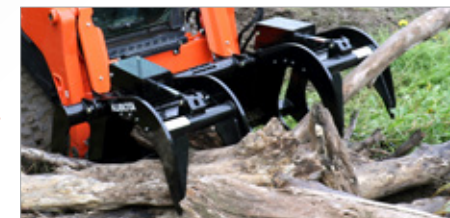
Two independent upper grapple jaws secure uneven loads.
