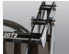
Large 1-1/4" diameter pivot pins provide extra strength.
