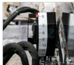
Depth indicator makes it easy to know depth of cut being made.
