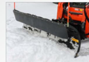
22° Blade oscillation helps the blade maintain contact while going over uneven surfaces.
