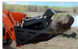
Two cylinder independent grapples help secure uneven loads.
