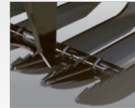
Two independent upper grapple jaws secure uneven loads.
