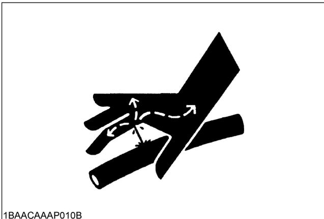
16. Fluid escaping from pinholes may be invisible. Use a piece of cardboard or wood to search for suspected leaks: do not use hands. Use safety goggles or other eye protection. If you get injured by escaping fluid, see a medical doctor at once. Serious infection or reaction will result if proper medical treatment is not administered immediately. This fluid can produce gangrene or severe allergic reaction.
