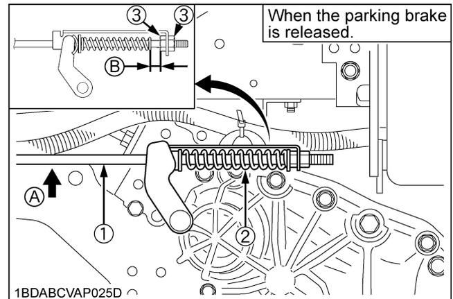
(1) Brake rod (2) Brake spring (3) Lock nut (A) "Hold the brake rod" (B) "Parking brake spring play"
