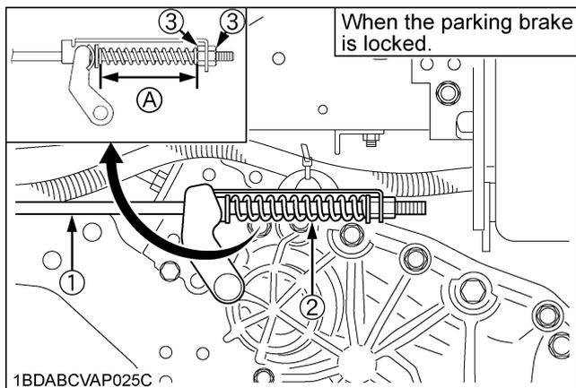
(1) Brake rod (2) Brake spring (3) Lock nut (A) "Parking brake spring length"
