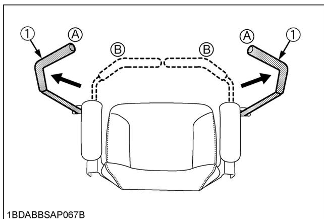
(1) Motion control levers (A) "NEUTRAL LOCK" position (B) "NEUTRAL" position (held by hand)
