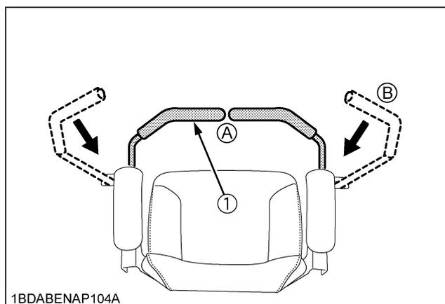
(1) Motion control levers (A) "NEUTRAL" position (B) "NEUTRAL LOCK" position
