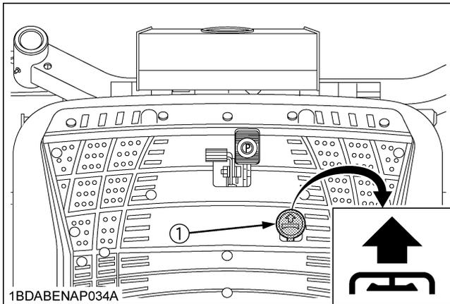
(1) Hydraulic lift control pedal "DOWN": Release the pedal
