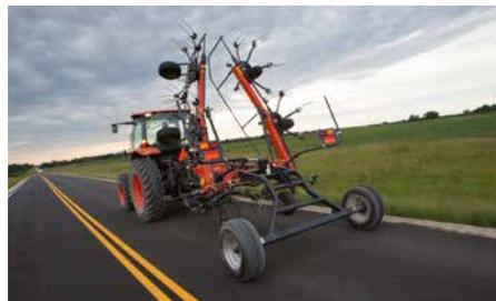
In transport position the weight of the carrier frame rests on the center part of the machine and the tractor drawbar.
