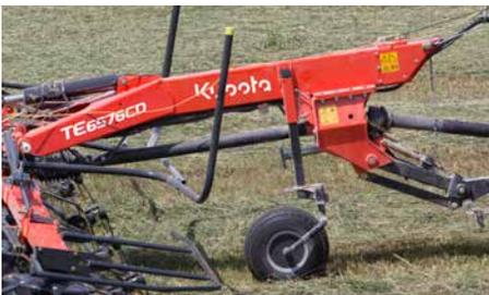
A third wheel allows for better tracking and more accurate tedding action. This wheel also helps adjust the tedding height.
