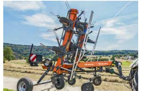
Standard running wheels of both models are extra wide 10.0/75 – 15.3 tyres with a generous track width of 8' (2.45m).
