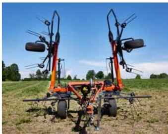
The tines are automatically leveled for added ground clearance when folding into the transport position.
