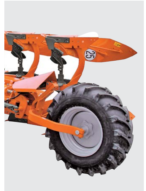
Very large wheel for the best flotation
