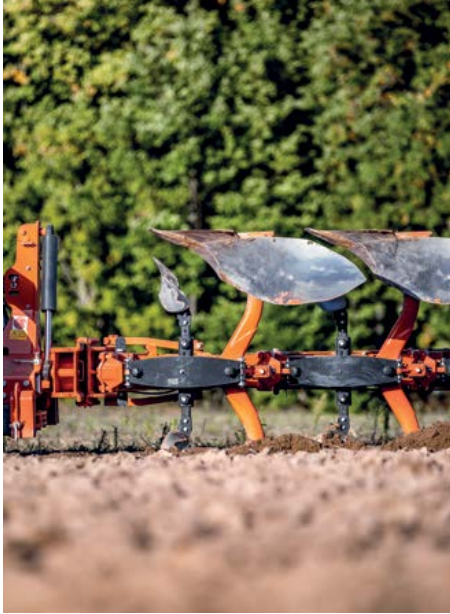
Aero-profile legs to avoid blockages in large residues
