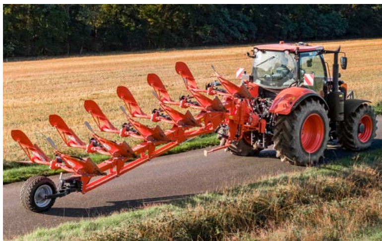
Rear mounted depth and transport wheel
