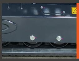
Maintenance time is reduced with permanently sealed and lubricated track rollers, and the grease type track tension system.
