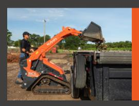
Vertical lift loader arms reach higher and further than the competition with a hinge pin height of 84.7" and a reach of 26" (at 45° dump angle).
