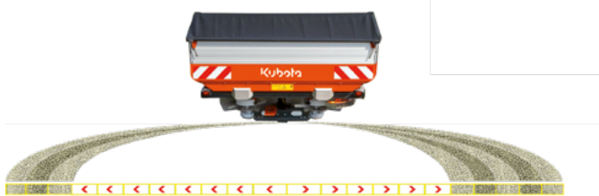
Switching off the sections outwards
