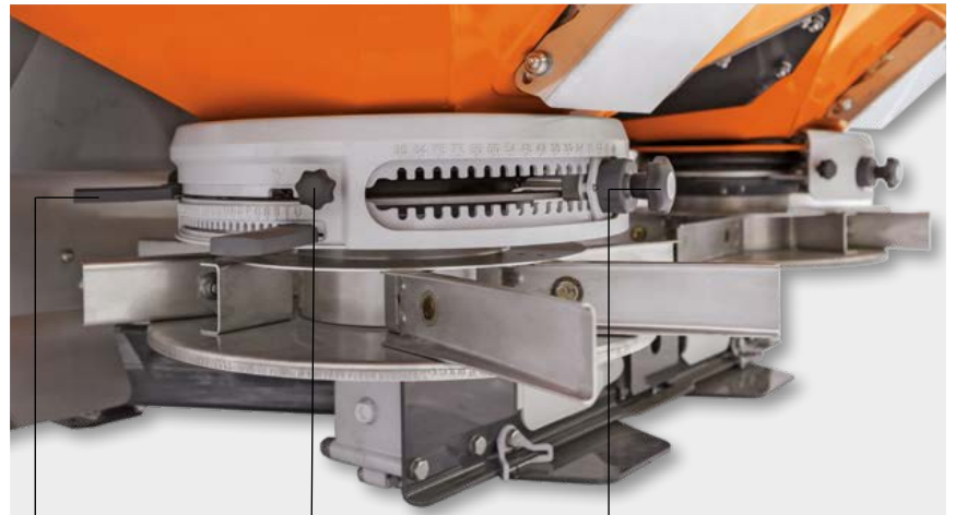
Fine application rate Discharge point Application rate
