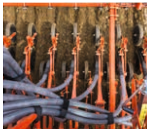
The Kubota CX-II coulters consist of two steel discs Ø325mm (Ø12 13/16") with 12.5cm (5") row spacing. Perfect depth control is ensured by the press wheels Ø250mm (9 13/16").
