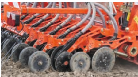
The Kubota CX-II coulters consist of two steel discs Ø325mm (Ø12 13/16") with 12.5cm (5") row spacing. Perfect depth control is ensured by the press wheels Ø250mm (9 13/16").
