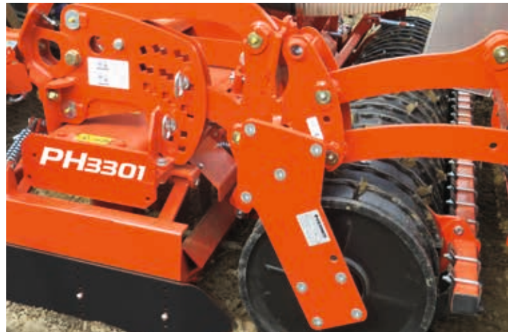
The coulters can easily disconnect to use the power harrow in solo operation e.g. on the headland.
