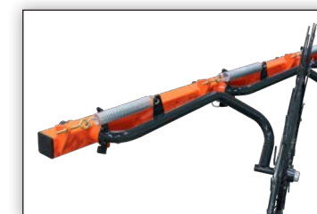
Individual floating rake wheels allows the wheels to closely follow the terrain
