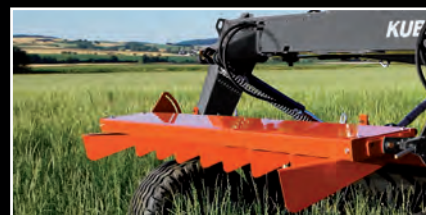
Dismount the two deflector doors and you are ready to mow.
