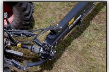
The swivel hitch headstock with reversible gearbox provides optimal maneuverability ability.
