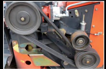
Adjustable rotor speed enables fuel saving and preservation of crop.
