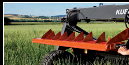
Changing from swathing to wide spreading is a one-man-job.
