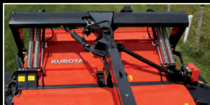
Kubota's DMC8536 and DMC8540 are fitted with 4 suspension springs for accurate ground pressure.
