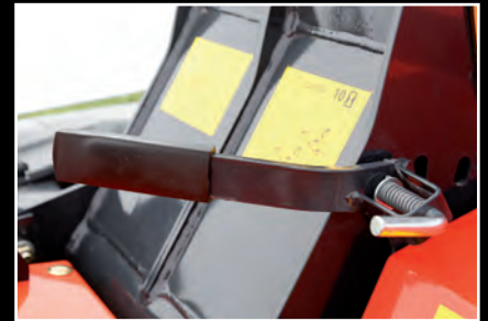
Easy adjustment of conditioning intensity.
