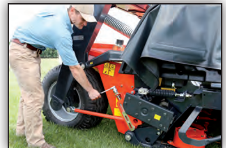
Easy adjustment of stubble height.
