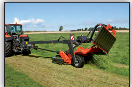
When placing the first swath, the belt is raised and hydraulically lowered for the second swath.
