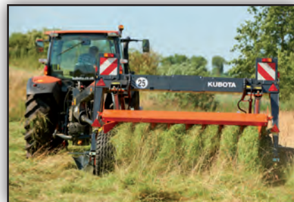
The crop is directed inwards, away from the unmowed crop.
