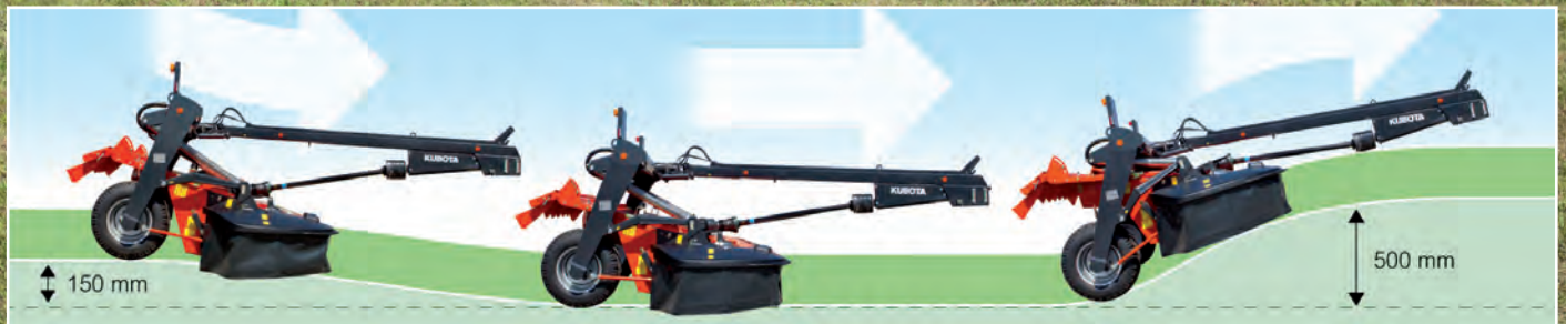
The suspension springs allow the mower to closely follow ground contours in uneven conditions. The cutting section can adapt 19.7inch (500mm) upwards and 5.9inch (150mm) downwards.
