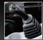
The U35-4 auto down-shift automatically shifts travel speed from high to low, depending on traction and terrain, allowing smoother operation when dozing and turning.
