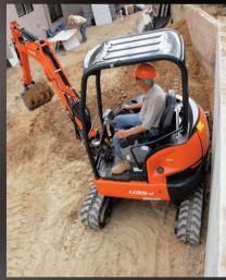
With its counterweight extending a mere 1.9 inches past the edge of the track, the U35-4's tight tail swing allows you to undertake operations where space is confined, and helps prevent costly damage to the engine hood and side panels. For added safety and improved operator visibility, the engine hood is set 5 inches inside the edge of the counterweight.
