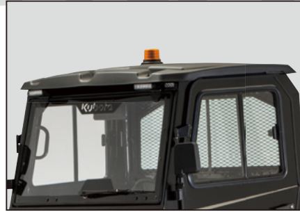
■ Plastic Canopy (RTV-X900 & RTV-X1120D only – Shown with VC5056 LED Strobe Light) VC5011
