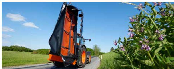
For transport the machine is folded hydraulically from the tractor cab to the vertical transport position well behind the tractor, ensuring a stable and steady transport.
