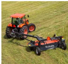
The swivel hitch headstock provides optimal maneuverability.
