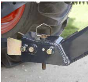
Kubota DM5032 and DM5040 are easy to connect to a tractor with a simple pin system.
