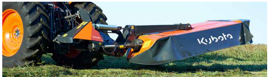
Lifting on headlands via hydraulic cylinder – ample ground clearance.
