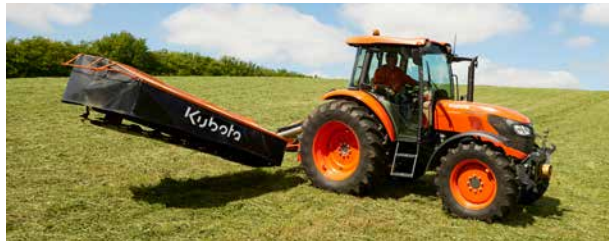
Lift on headlands via a hydraulic cylinder – no use of the 3-pt hitch is needed.
