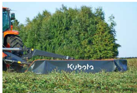
The centre suspended design enables fast and precise adaptation to ground contours.
