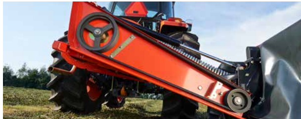
Four v-belts ensure excellent transfer of power.
