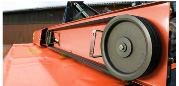
By switching driveline pulleys changing from standard PTO speed of 1000 rpm to 750 rpm is possible.
