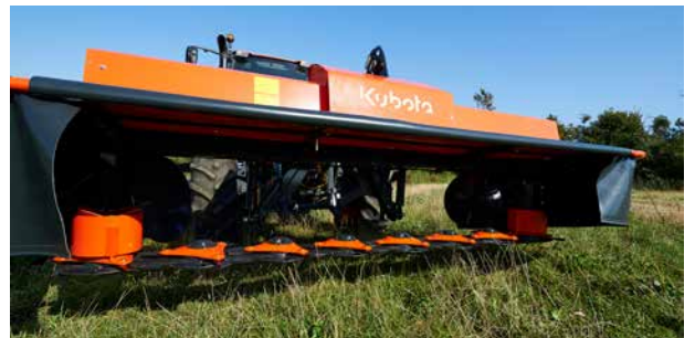
Easy access to the cutterbar with foldable front and side guards.
