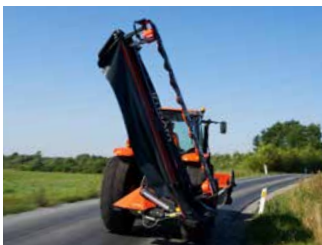
Up to 125° vertical transport position for excellent weight distribution.
