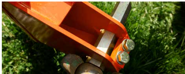
The linkage pins are easily adjusted to match the tractor width, which enables the mower to cut to its' full working width.
