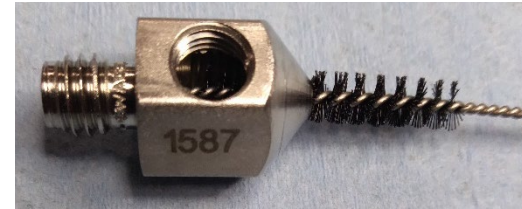
Brush inside the nozzle bore (both ends), female thread, and inside the central cavity of the part
