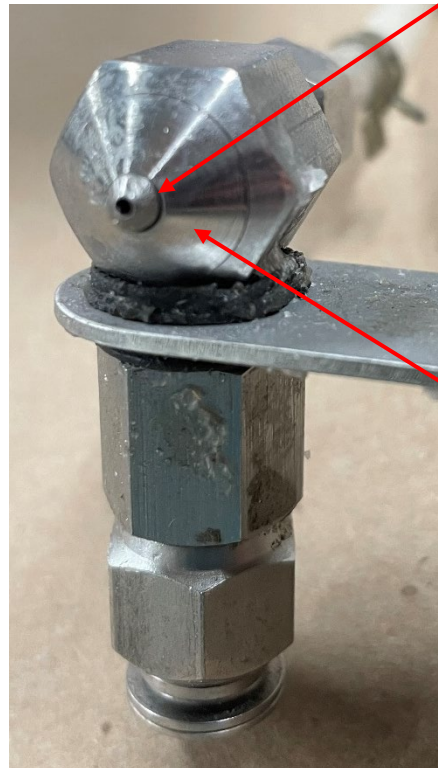
Functioning nozzle after a sealing job.
