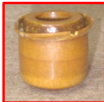
Leaking Ferrule – Installed and tightened backward in the nozzle body
