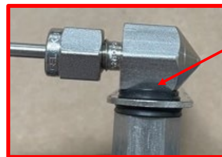
Overtightened Q-Ring – the inner seal surface is beginning to slide up the side of the nozzle body (leaks)
