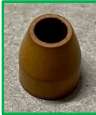
Functional Ferrule – smooth surfaces, clean edges
