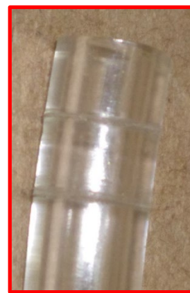
Gouged surfaces on the flexible tube (area inserted into the PTC)
