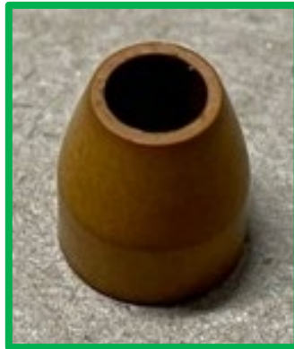
Functional Ferrule – smooth surfaces, clean edges
