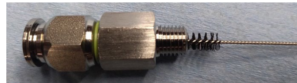
Brush the interior of the air inlet fittings (both ends)
