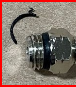
Cut or Damaged O-Ring (internal and external)
