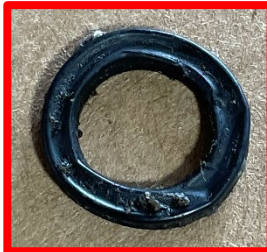
Damaged Q-Ring (distortion from over-compression and debris from incomplete cleaning)
