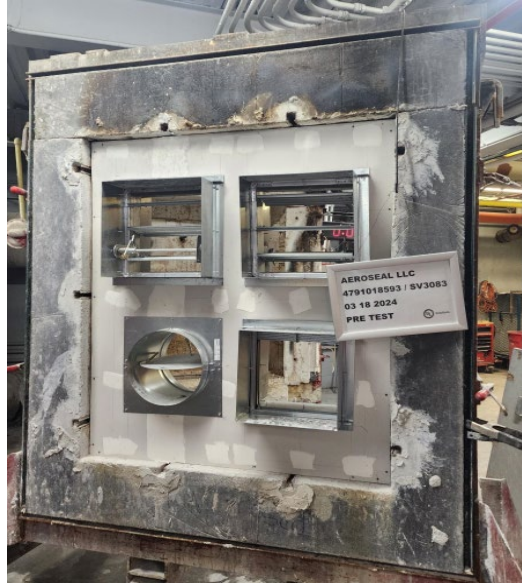
UNEXPOSED SIDE OF TEST ASSEMBLY PRE-TEST
