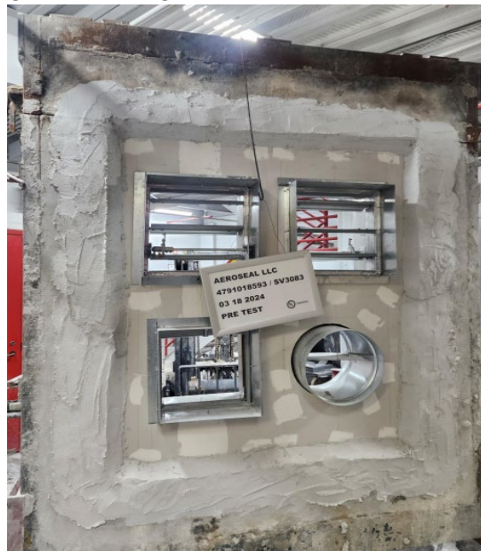
EXPOSED SIDE OF TEST ASSEMBLY PRE-TEST
