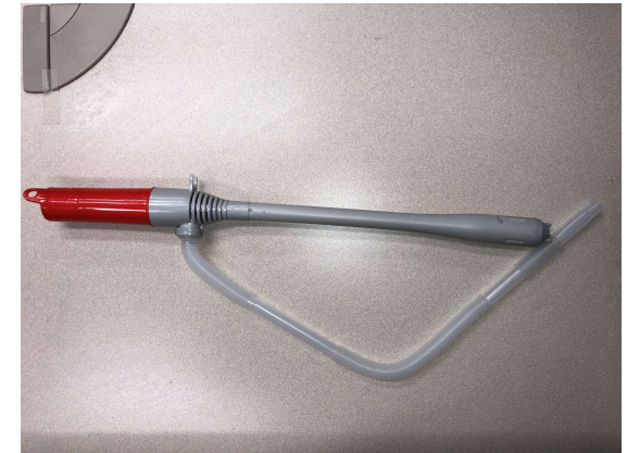
Sealant Transfer Pump
