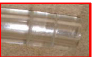
Gouged surfaces on the flexible tube (area inserted into the PTC)
