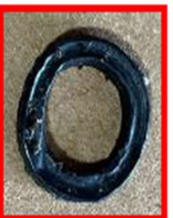
Damaged Q-Ring (distortion from over-compression and debris from incomplete cleaning)
