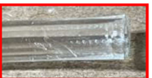
Gouged surfaces on the flexible tube (area inserted into the PTC)
