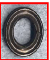
Damaged Q-Ring (Cut by twisting nozzle after assembly)
