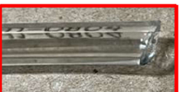
Angled cut on tube end
