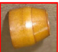
Leaking Ferrule: Sharp ridge at end of tapered surface, chipped leading edge (excessive compression from seal nut)
