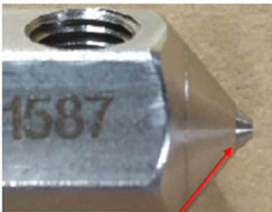
Adjust Insert Tube stick-out so the taper matches the nozzle.
