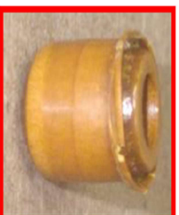
Leaking Ferrule: installed and tightened backward in the nozzle body
