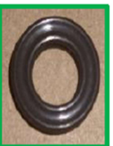
Functional Q-Ring (round, clean, all surfaces intact)
