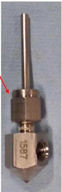
Tighten seal nut: finger tight + 1/4 turn MAX
