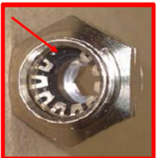
PTC Missing Retention Teeth (Tube pulled out without fully compressing collar)
