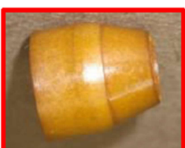
Leaking Ferrule: Sharp ridge at end of tapered surface, chipped leading edge (excessive compression from seal nut)
