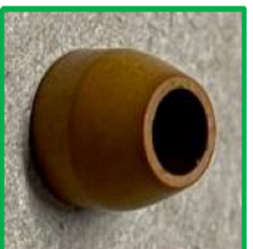
Functional Ferrule: smooth surfaces, clean edges
