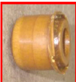
Leaking Ferrule: installed and tightened backward in the nozzle body
