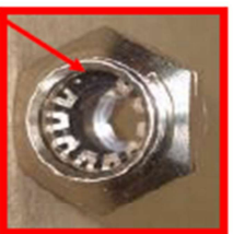
Damaged retention teeth
