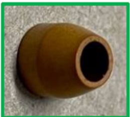
Functional Ferrule: smooth surfaces, clean edges
