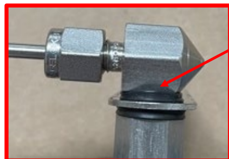
Overtightened Q-Ring – the inner seal surface is beginning to slide up the side of the nozzle body (leaks)
