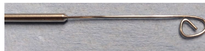
Ram rod for the interior of the insert tube
