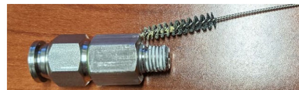
Brush the Exterior of the air inlet fittings
