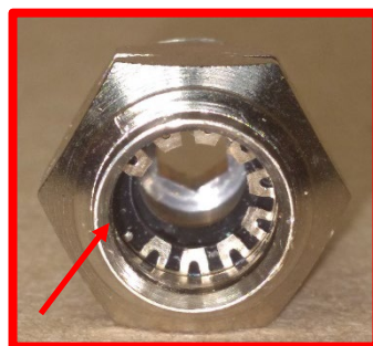
Damaged retention teeth
