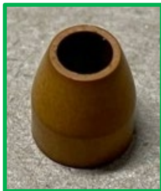
Functional Ferrule – smooth surfaces, clean edges
