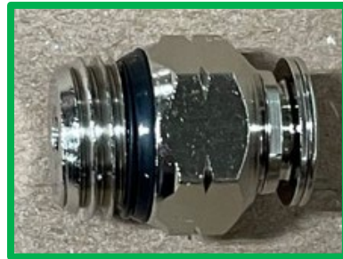
Clean, Functional PTC – no damage and release collar moves freely
