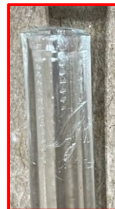
Gouged surfaces on the flexible tube (area inserted into the PTC)
