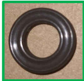
Functional Q-Ring (round, clean, all surfaces intact)
