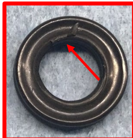
Damaged Q-Ring (Cut by twisting nozzle after assembly)
