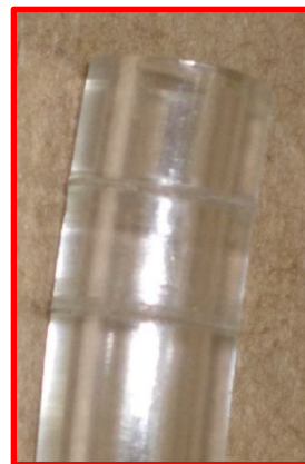
Gouged surfaces on the flexible tube (area inserted into the PTC)
