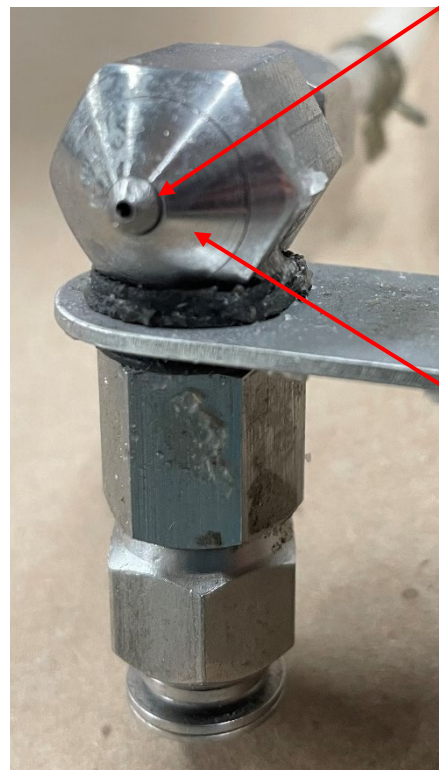
Functioning nozzle after a sealing job.
