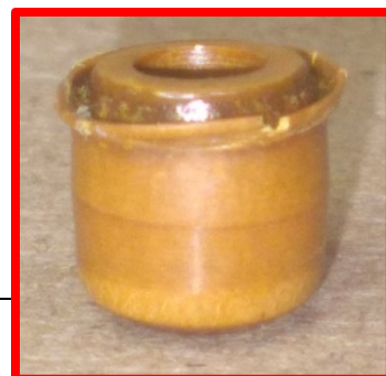
Leaking Ferrule – Installed and tightened backward in the nozzle body
