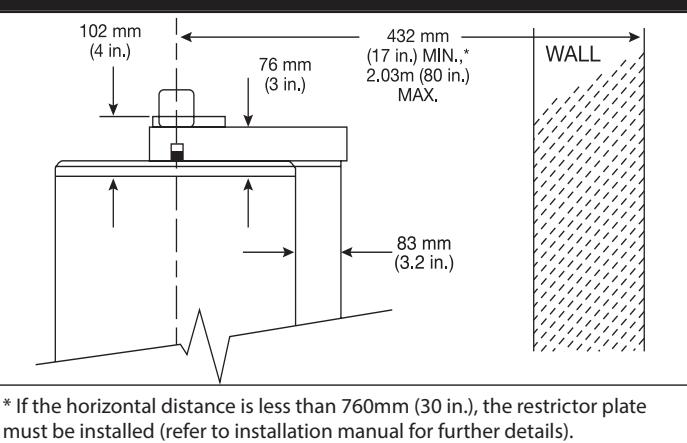
\* If the horizontal distance is less than 760mm (30 in.), the restrictor plate must be installed (refer to installation manual for further details).
