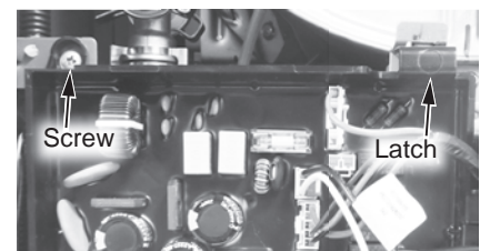
Figure 263 - Control board location
