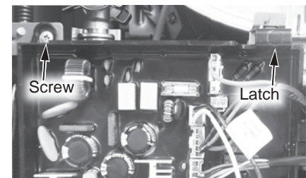
Figure 158 - Control board panel location
