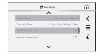
Historical data is stored in the FMM. If this board is removed or damaged during servicing the historical data will be lost and heater will no longer operate. The FMM should never be replaced unless directed by Technical Support.
