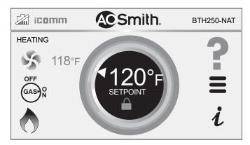
Figure 64. Tank Temperature Set Point
