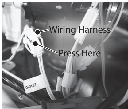
Figure 73 - Wiring harness location
