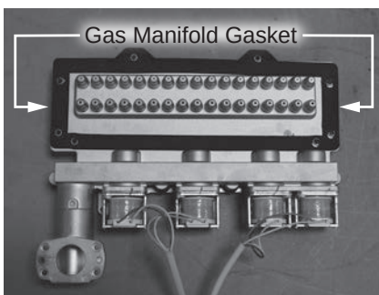
Figure 128 - Replacing gas manifold gasket
