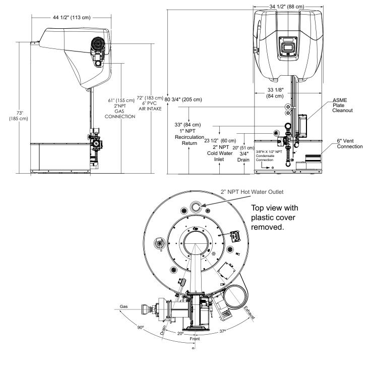
Electrical characteristics-120V-60Hz A.C., 5.0 A "A" in model represents ASME construction Propane gas models available Dimensions and specifications subject to change without notice in accordance with our policy of continuous product improvement.
