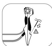
Dip the tip of endoscopy biopsy forceps in water-soluble medical-grade lubricant and run through the channel until the tip comes out of the distal end of the scope. Open and close the forceps. Ensure the forceps are closed, and then remove them from the device. Forceps should go through smoothly. Place forceps on tray/package until ready for use.
