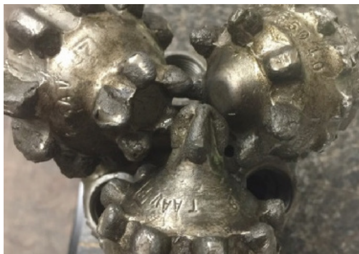
Roller cone Bit #1 - Drilled out 70 Obsidian® frac plugs with no short-trip
