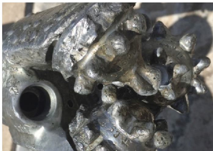
Roller cone Bit #2 - Drilled out 54 Obsidian® frac plugs in one short-trip after 30 Obsidian® plugs
