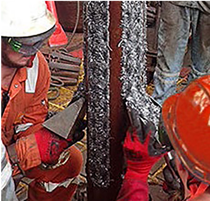
PowerMag® magnet being cleaned on rig floor after milling run with cleaning tool
