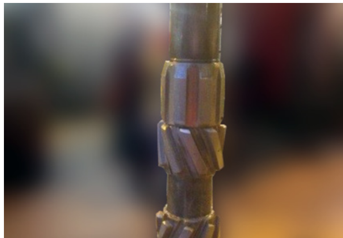
Well No. 2 – The 9 5/8 in. Drill Tech® scraper's condition after drilling 341 m (1,119 ft) of open hole
