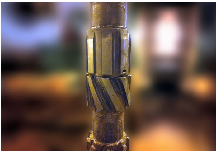
Well No. 1 – The 9 5/8 in. Drill Tech® scraper after drilling tieback, shoe track, and 81 m (266 ft) of open hole
