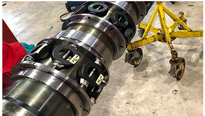
Metallic specimens mounted on material test sub
