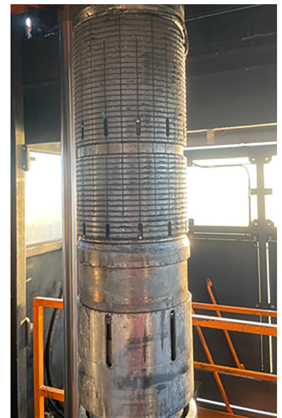
X-Trieve™ HC AHC packer recovered from the well
