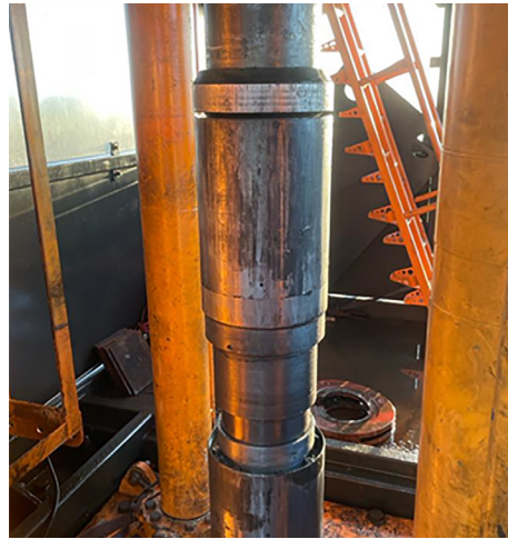
Material test sub recovered from the well.
