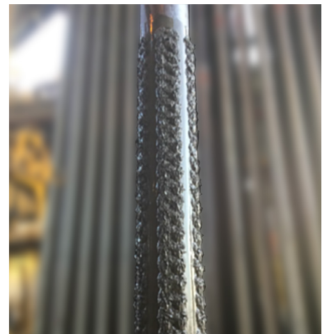
186 lbs of ferrous debris collected during whipstock run
