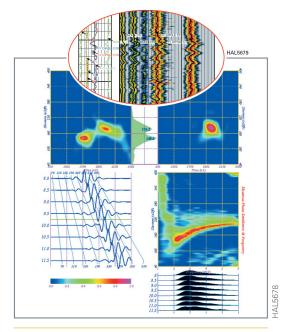
This is an example of a semblance diagnostic plot of the waveform data from the eight waveforms. In the circle is a section of a log showing monopole P-wave slowness and semblance quality, monopole refracted shear-wave slowness and semblance quality, X-X dipole slowness and semblance quality, and Y-Y dipole slowness and semblance quality.
