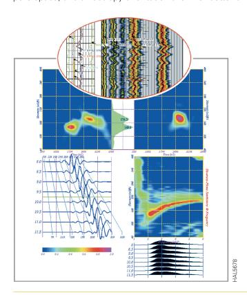
This is an example of a semblance diagnostic plot of the waveform data from the eight waveforms. In the circle is a section of a log showing monopole P-wave slowness and semblance quality, monopole refracted shear-wave slowness and semblance quality, X-X dipole slowness and semblance quality, and Y-Y dipole slowness and semblance quality.
