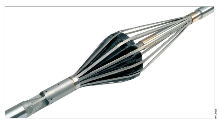
Halliburton's Diverter Basket Flowmeter (DBT) is an ideal way to determine fluid velocity for vertical or deviated wells. The DBT is designed to provide accurate measurements from a stationary position for low or medium flow-rate wells. As part of an Ultrawire™ toolstring, it operates in tandem with other Ultrawire tools, increasing the coordination between logging tools and applications. An extender flow tube can also be attached, enabling its use with a Fluid Density Radioactive (FDR) tool.
