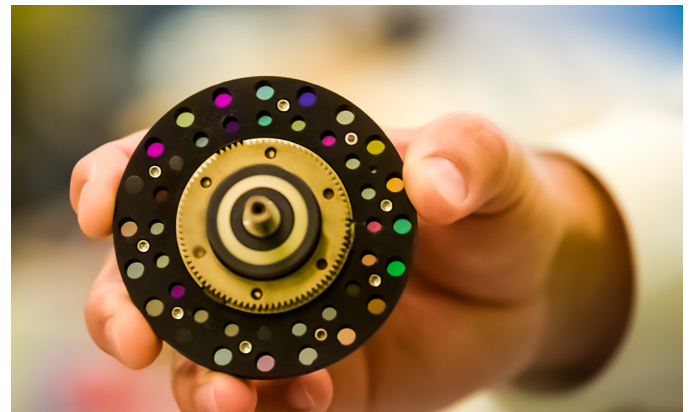
The ICS20 will take up to 20 ICE Core® measurements downhole using a rotating wheel of selected sensors.
