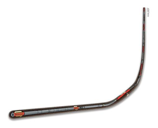
The Halliburton Toolpusher™ drillpipe-conveyed logging system helps acquire premium-quality data in highly deviated wells.
