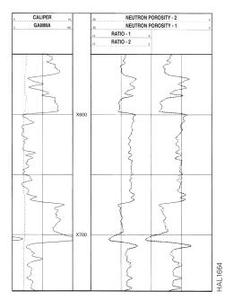
In this LOGIQ® DSN II™ log example, the subject well was logged twice. The resulting near/far ratio curves and the calculated porosity curves are overlaid to illustrate the high repeatability of DSN II tool porosity measurements.
