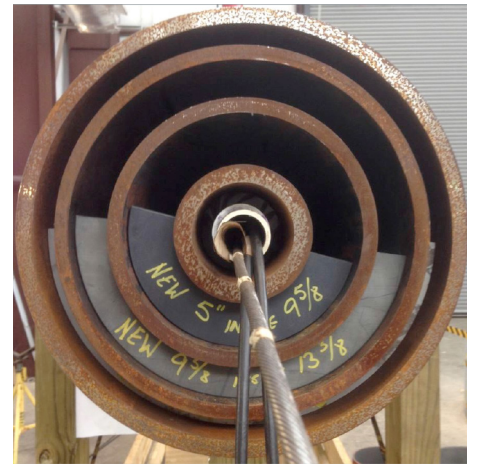
The Electromagnetic Pipe Xaminer® V tool has been thoroughly tested in multiple casing scenarios, helping to ensure that the technology is characterized and delivers an accurate metal-loss assessment. The above image corresponds to a four-casing setup, including 5-in. OD, 9 5 / 8 -in. OD, 13 3 / 8 -in. OD, and 16-in. OD casings.
