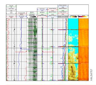
Cement evaluation and casing inspection logs from the BSAT $^{\text{\tiny{M}}}$  and CAST-XR $^{\text{\tiny{M}}}$  services are combined to provide the optimum zonal isolation and well integrity answers in high-thickness casings.
