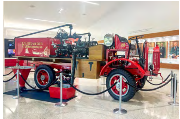
Halliburton oil well cementing truck from the early 1900s.
