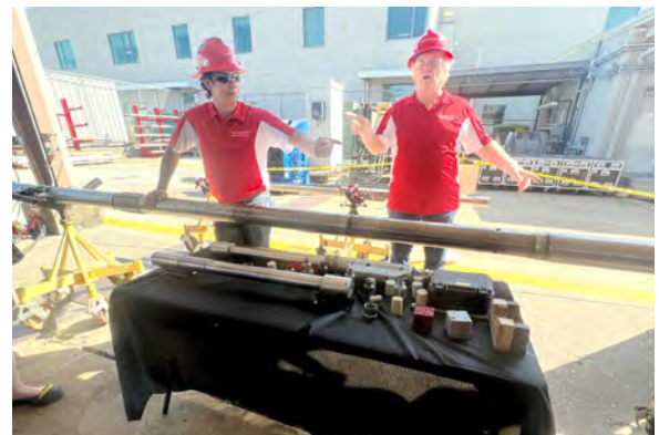
Their expert operators show the rotary sidewall coring tool on display.
