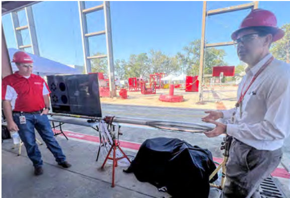
A PLT tool on display works in a water-filled pipe to show the tool's capabilities and how previous challenges have been addressed in this version. The screen on the left side showed us the real-time readings.
