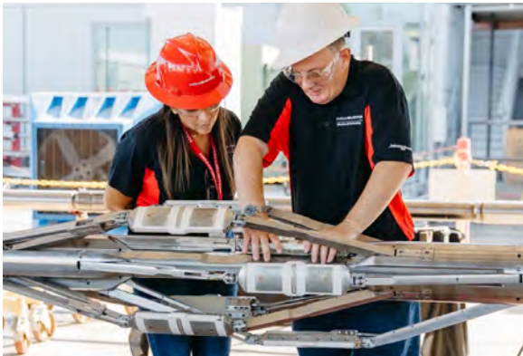
Eglee Lopez and Peter Barrett show how the StrataXaminer borehole image tool can adjust for challenging borehole conditions.
