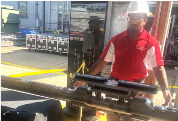
Gibran Hashmi shows the pads used with the formation tester and sampling tool depending on reservoir conditions and challenges.
