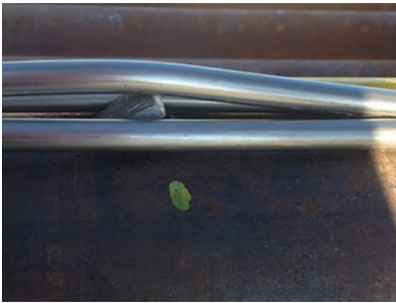
Slow blade movement prevents damage to control lines or TEC cables
