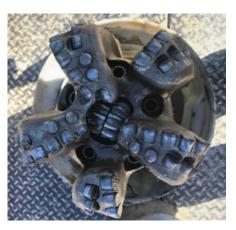
Utilizing Crush & Shear hybrid bit technology enabled the operator to successfully complete the curve section of the subject well in just one run – achieving an ROP of 25 feet/hour (7.6 meters/hour), beating the ROP in the offset wells by over 5 feet/hour (1.5 meters/hour). Additionally, this solution reduced the cost of the interval, saving the customer over USD 120,000.
