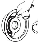
2. Pull inflation valve housing to release air.
