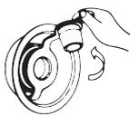
(1b) If valve housing already inserted inside exhaust hole, pull valve cap to open.
