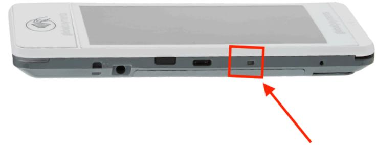
The LED indicator is on the side of the S1000E terminal, as shown above. The following coloured lights indicate the terminal's power status:
