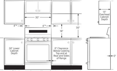
\* Side clearance above cooking surface to any objects, i.e., wall.
