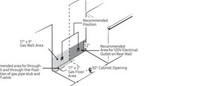
Recommended area for through-the-wall and through-the-floor connection of gas pipe stub and shut-off valve.
