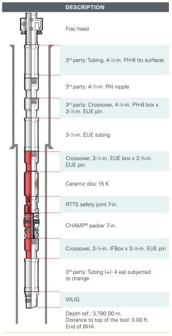
Frac string redesigned to include tubing with higher elasticity to mitigate usage of the slip joint.
