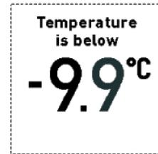
Temperature below zero can damage the sensor. The recommended operating temperature of the sensor is 0 °C to 50 °C (32 °F to 122 °F).
