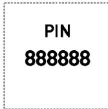
Six-digit pin code displayed for wirelessly connecting the device with your smartphone to the Aranet4 app via Bluetooth.
