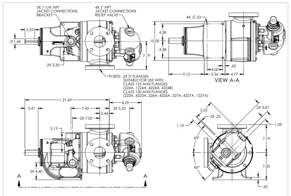
STANDARD MODELS: LS224A, LS1224A, LS4224A, LS4224B, LS223A, LS4223A, LS226A, LS4226A, LS227A, LS4227A, LS1227A
