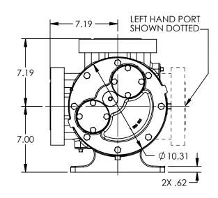
MODELS WITH OPTIONAL FLANGED PORTS: LS123C, LS4123C, LS127C, LS1127C, LS4127C
